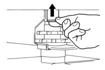
Pull out the Brightness Select Lever and slide it to a position appropriate for the type of the Projection Lens loaded in the machine.
